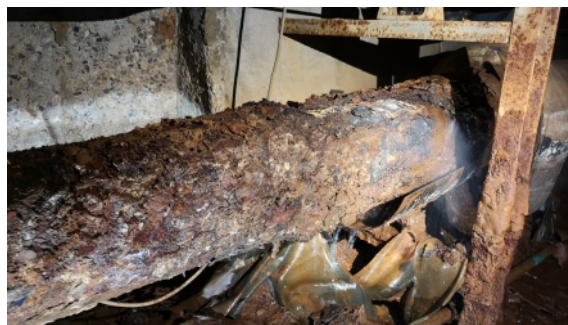
Section two of the pipe was breached underneath
