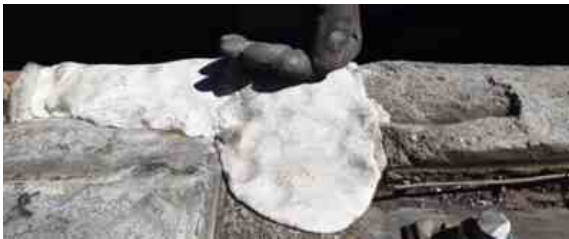
Effluent was escaping from both ends of a failed pipe repair clamp, seen in the centre of the pipe.
