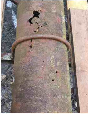
Corrosion had breached the pipe in several places
