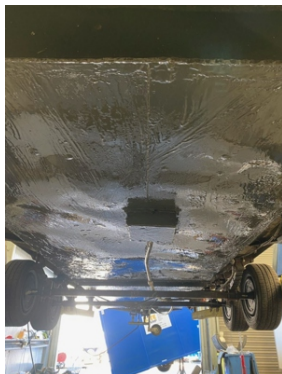
AB Original Black Epoxy Putty filled in all holes
