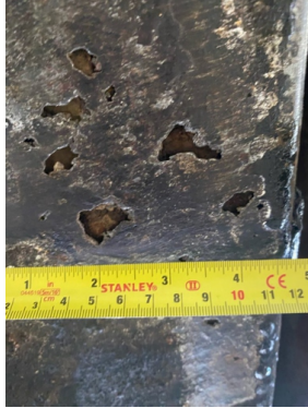
Wastewater holding tanks underneath the two trailers were suffering from corrosion and multiple holes
