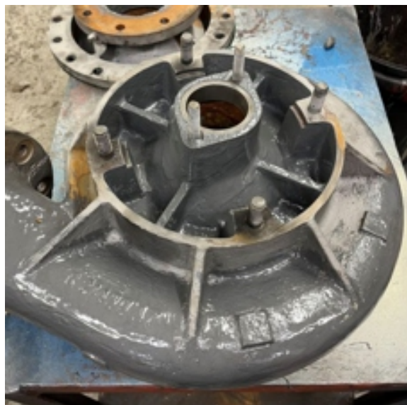
Superfast Steel sealed the pinholes in the casing and a 3mm coating of Liquid Metal provided thorough protection against future corrosion
