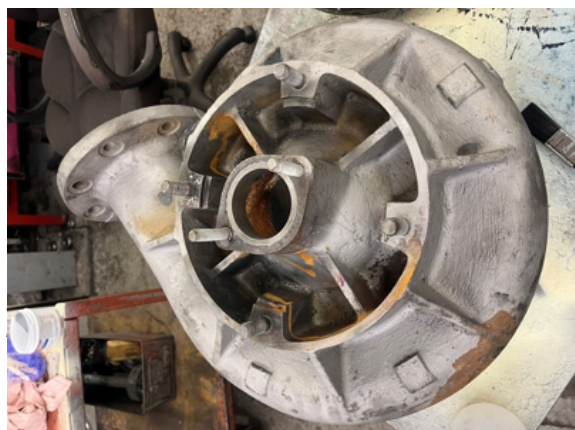
Once shot-blasting was completed and the pump pressure tested, multiple pinhole leaks were found
